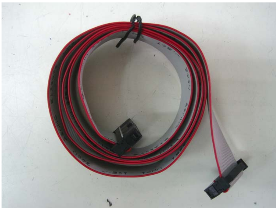
View of the Display Cable
